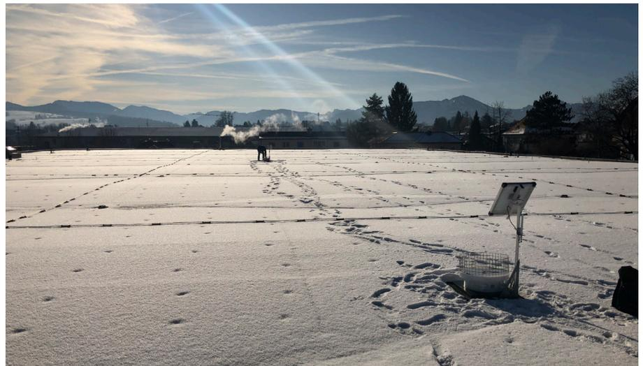
because of roof structures or fire protection walls. These variations in the snow load or backwater can only be recorded by a large number of measuring points like the envitron snow measurement system. So, in case of an emergency, the roof clearance can be initiated and people can be evacuated in time and lives be saved.
